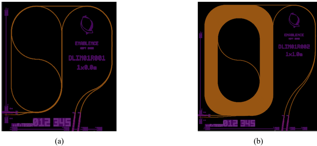
Figure 2. Examples of k-clock systems based on delay lines and interferometers for (a) GHz frequency systems, and (b) MHz frequency systems. The compact form factor allows for a wide range of customized k-clocks to be realized in PLCs within a small footprint.
